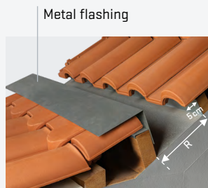
Exemple of an internal gutter using flashing
